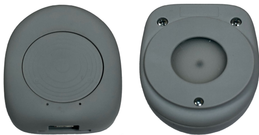
FIGURE 1. The photography of the sensor; outer part on the left, and inner part (directed to the body) on the right.
