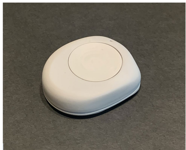
Fig. 1 Photography of the sensor with dimensions of 33 \times 39 \times 13 mm and 18 g of weight
