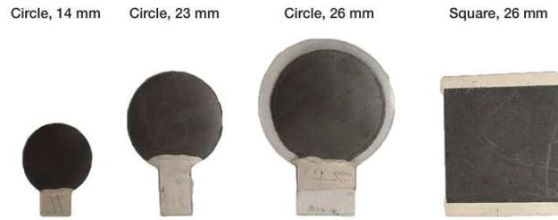
Fig. 1: Photograph of the investigated graphene electrodes.
