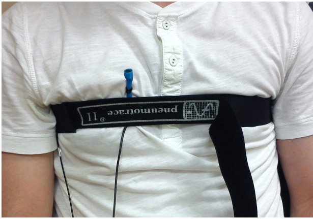
Fig. 1. Positioning of the microphone and MLT1132 Piezo Respiratory Belt Transducer
